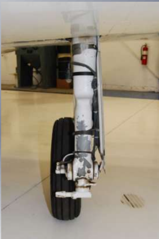
Left main landing gear
